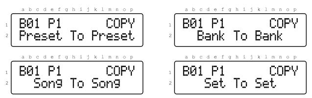
To move/scroll the Preset, Bank, Song or Set copy, press the **DEC**→(**DOWN**) or **INC**→(**UP**) switch. And press **ENTER(EDIT/2ND)** switch.
